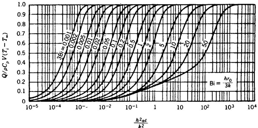
Fig. 43.11 Internal energy change as a function of time for a sphere of radius  $r_0$ .<sup>4</sup> (Used with the permission of McGraw-Hill Book Company.)
