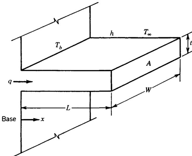
Fig. 43.2 Heat transfer by extended surfaces.
