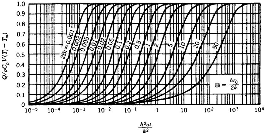
Fig. 43.8 Internal energy change as a function of time for an infinite cylinder of radius  $r_0$ .<sup>4</sup> (Used with the permission of McGraw-Hill Book Company.)
