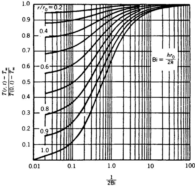
Fig. 43.7 Temperature distribution in an infinite cylinder of radius  $r_0$ . (Adapted from Heisler.<sup>3</sup>)
