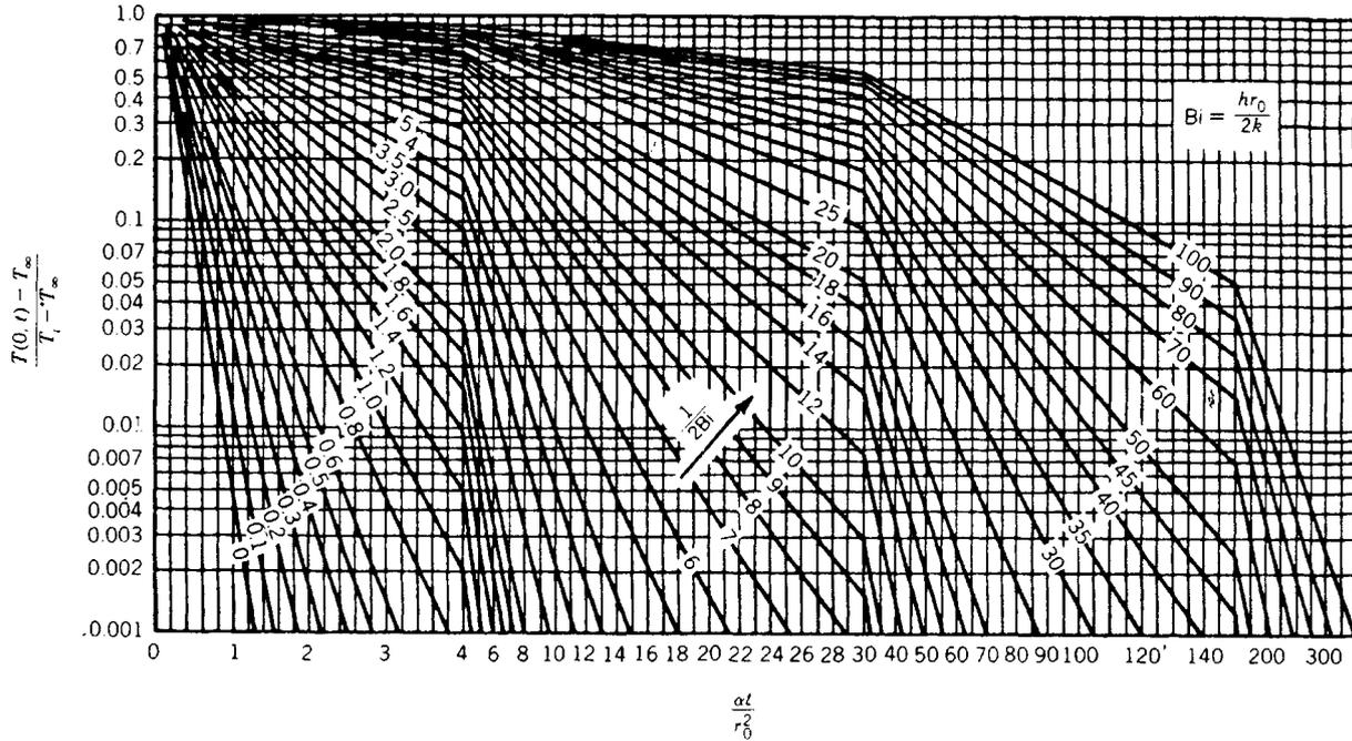
**Fig. 43.6** Centerline temperature as a function of time for an infinite cylinder of radius  $r_0$ . (Adapted from Heisler.<sup>3</sup>)
