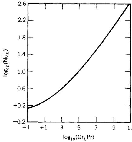
**Fig. 43.13** Free convection heat-transfer correlation for heated vertical plates and cylinders. Adapted from Ref. 14. (Used with permission of McGraw-Hill Book Company.)
