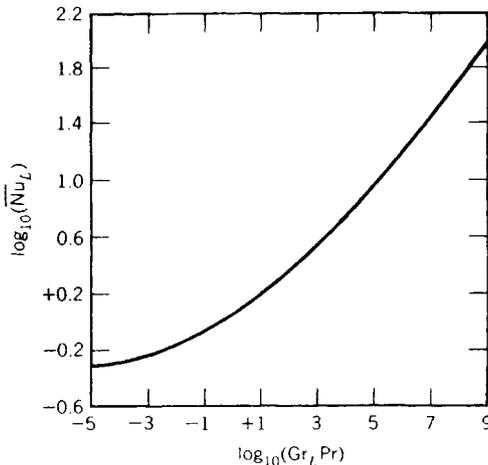
**Fig. 43.14** Free convection heat-transfer correlation from heated horizontal cylinders. (Adapted from Ref. 14. Used with permission of McGraw-Hill Book Company.)
