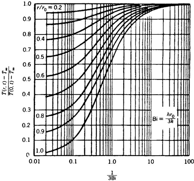
Fig. 43.10 Temperature distribution in a sphere of radius  $r_0$ . (Adapted from Heisler.<sup>3</sup>)
