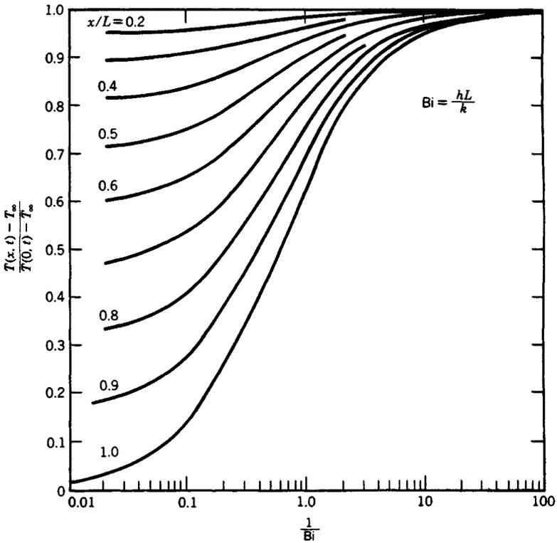
Fig. 43.4 Temperature distribution in a plane wall of thickness  $2L$ . (Adapted from Heisler.<sup>3</sup>)
