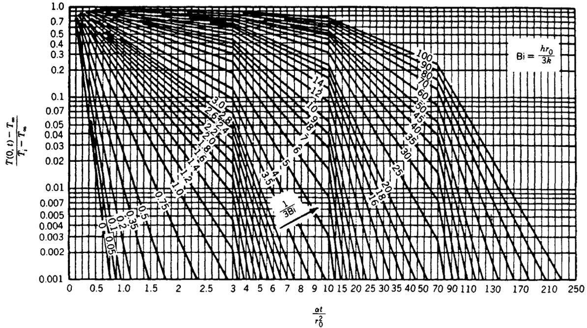
Fig. 43.9 Center temperature as a function of time in a sphere of radius  $r_0$ . (Adapted from Heisler.<sup>3</sup>)
