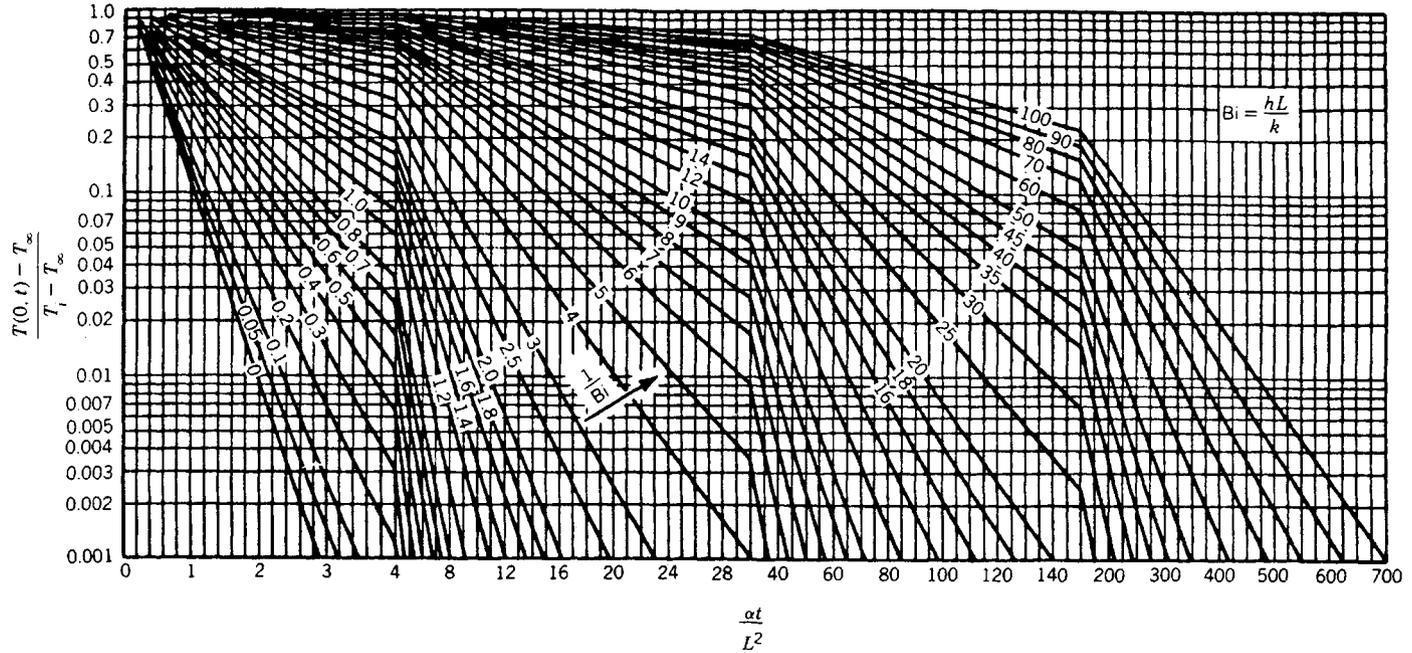
Fig. 43.3 Midplane temperature as a function of time for a plane wall of thickness  $2L$ . (Adapted from Heisler.<sup>3</sup>)
