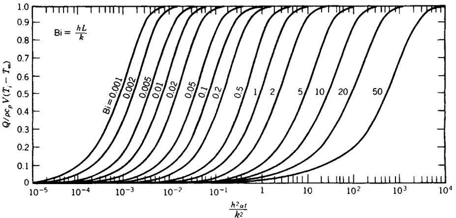
Fig. 43.5 Internal energy change as a function of time for a plane wall of thickness  $2L$ .<sup>4</sup> (Used with the permission of McGraw-Hill Book Company.)
